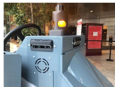
Right side : Laser on top of the light, right and center depth cameras.
