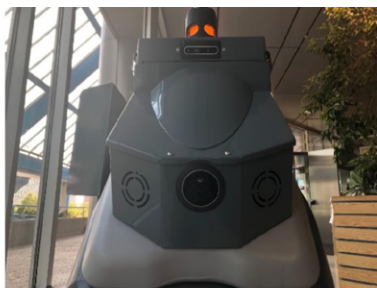
Front side : Laser on top of the light, center depth camera and bottom laser camera.
