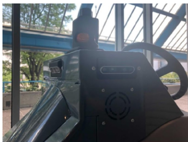
Left side : Laser on top of the light, left and center depth cameras
