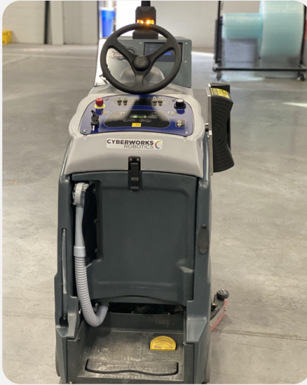
THE SCRUBBER ENHANCED WITH A CYBERCUBE KIT CONTAINING THE ELECTRONICS AND COMPUTER ALLOWING AUTONOMOUS NAVIGATION.
